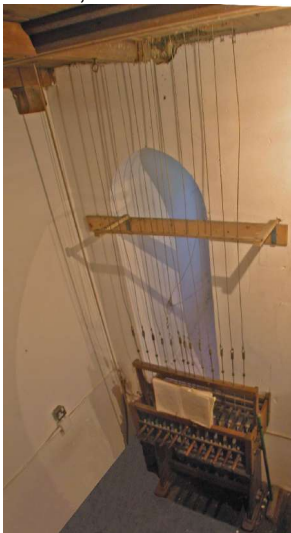
Above, is the first floor where the cables from the simple bell pulling control, pass upwards through the ceiling. There are twelve levers in a row, each is pushed down to strike its bell. A thirteenth lever, above the row, acts as the "black" key on a piano.
