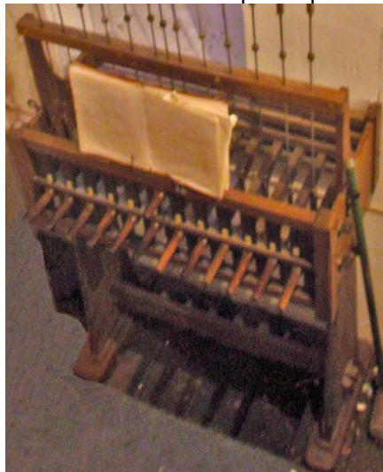
Above, is the first floor where the cables from the simple bell pulling control, pass upwards through the ceiling. There are twelve levers in a row, each is pushed down to strike its bell. A thirteenth lever, above the row, acts as the "black" key on a piano.
